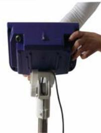
Step 4: After connecting load cell connector to load cell port, the installation is completed.
